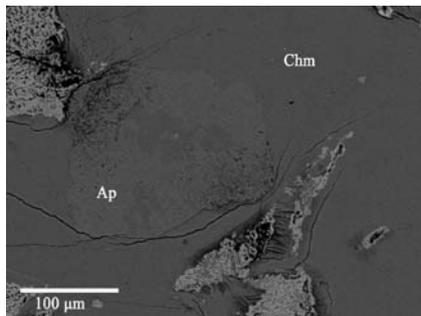
**fig 3.** BSE image of an apatite crystal located at the core of a chamosite ooid occurring at the third ironstone horizon. (Chm: chamosite; Ap: apatite).
