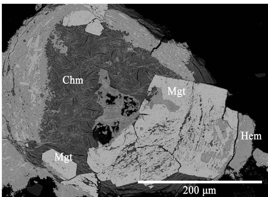
fig 1. Backscattered electron image (BSE) of an ooid of the first ironstone horizon, showing martitization. (Chm: chamosite; Mgt: magnetite and Hem: haematite).
