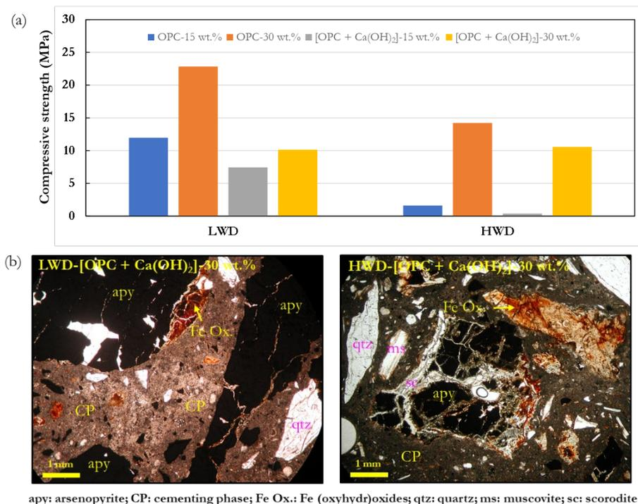
**Fig 1.** (a) Compressive strength development of cemented mine wastes. (b) Microscopy images of cemented mine wastes.
