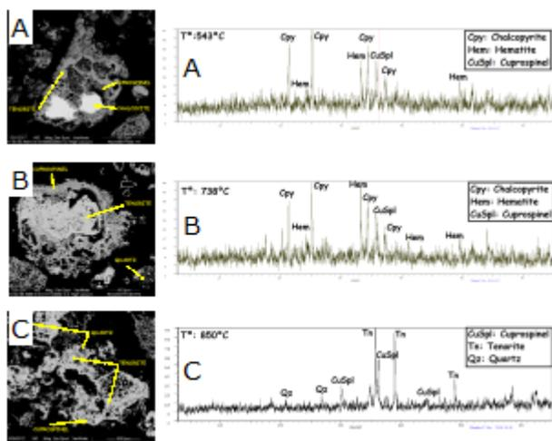
Fig 3: BSE images (left) and diffractograms (right) of TGA residues at indicated temperatures. A and B at 45% Oxygen mixture, C at 21%  $O_2$ .
