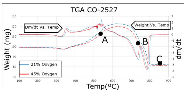
Fig 2. TGA graph representing mass (main axis) and  $dm/dt$  (secondary axis) vs. temperature under two oxidizing conditions.
