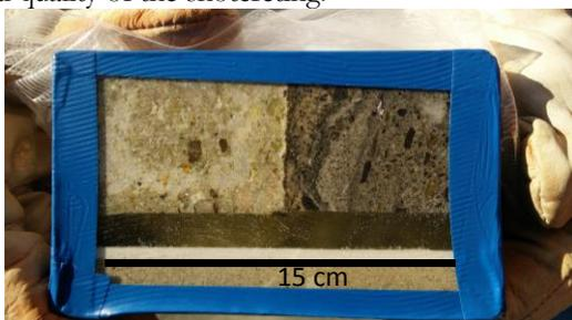
**Fig 1.** Undisturbed 13 years bentonite (left)/ concrete (right) contact.
