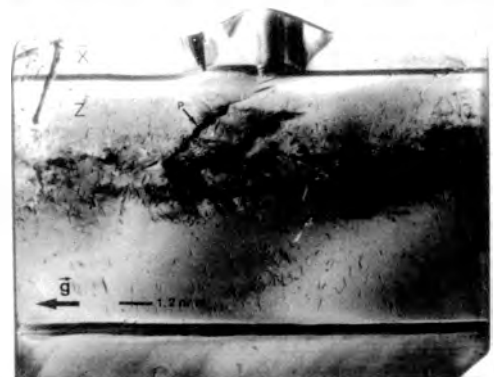
Fig. 4. traverse topograph corresponding to the external Z-plate showing the invisibility of (0\bar{1}11) composition planes in the Z growth sectors. 0\bar{1}10 reflection.
